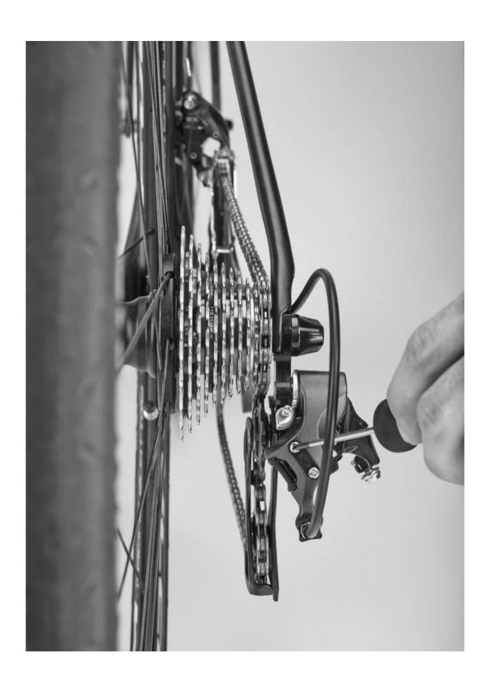
With the gear cable disconnected, gently pedal forwards until the chain drops onto the smallest sprocket. Find the screw towards the back of the derailleur marked H (for high). This is typically a cross-head, but some derailleurs use hex-head screws instead.
