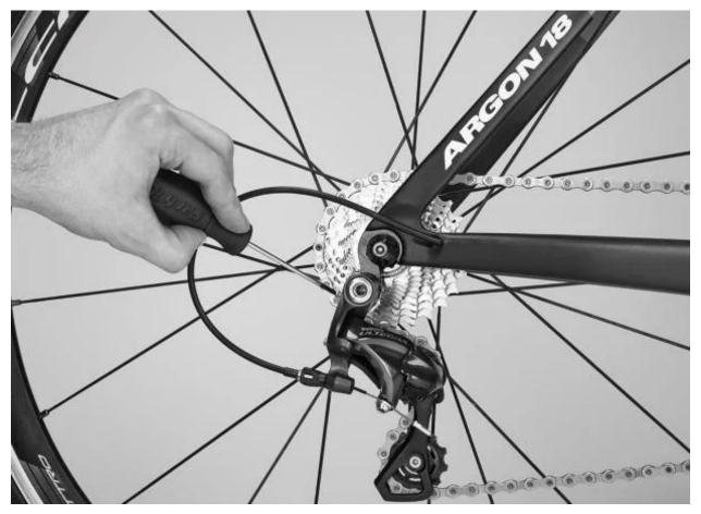
With the chain still on the largest sprocket, it's time to adjust the B-tension screw – find it on the upmost part of the derailleur, next to where it mounts on the frame.
