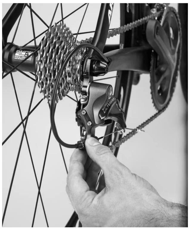
Use the barrel adjuster to fine-tune its position. Turning the adjuster anticlockwise increases tension on the cable, bringing the derailleur
