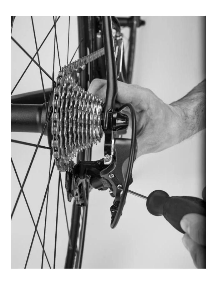
Shift into the largest sprocket. Find the screw marked L (below the H screw). It dictates how far towards the wheel the derailleur can move (the lower limit).
