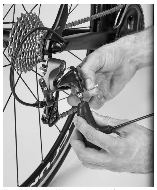
Turn the barrel adjuster on the derailleur clockwise until it is almost fully screwed in. Select
